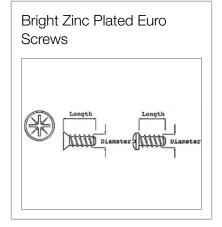
Metric Dia x L (mm) Head SY0168 6.3 x 11 Counter Sunk SY0194 6.3 x 13 Counter Sunk SY0197 6.2 x 10.5 With Collar SY0607 6.3 x 16.2 Pozi SY0771 6.3 x 13 Pozi
